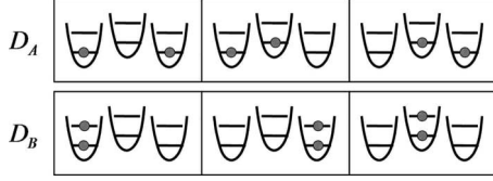
FIG. 4. Possible configurations of the TQD system with two holes. The circles represent holes and the separation between two levels in the same dot is the on-site Coulomb repulsion energy U . Configurations with no doubly occupied dot belong to D_A and configurations with a doubly occupied dot belong to D_B . The energy levels of the second dot are shifted by \Delta by applying appropriate voltages to the gate electrodes. Configurations in D_B have much higher energy than configurations in D_A due to the large on-site Coulomb repulsion energy.
